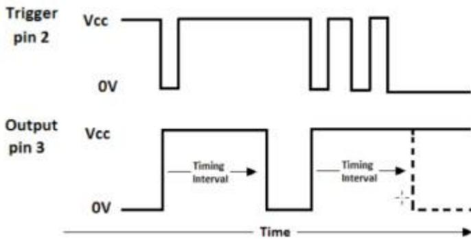
Figure 3: Timing diagram for 555 in monostable mode.
