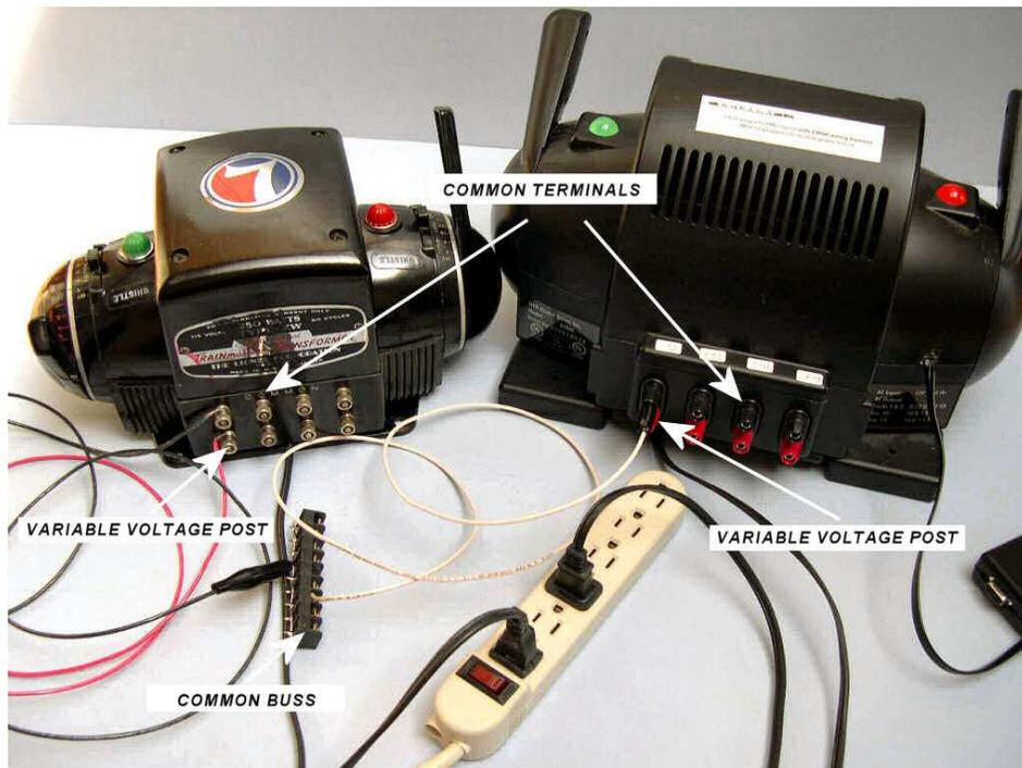
Figure 1 – ZW and Z400 connected to common buss
