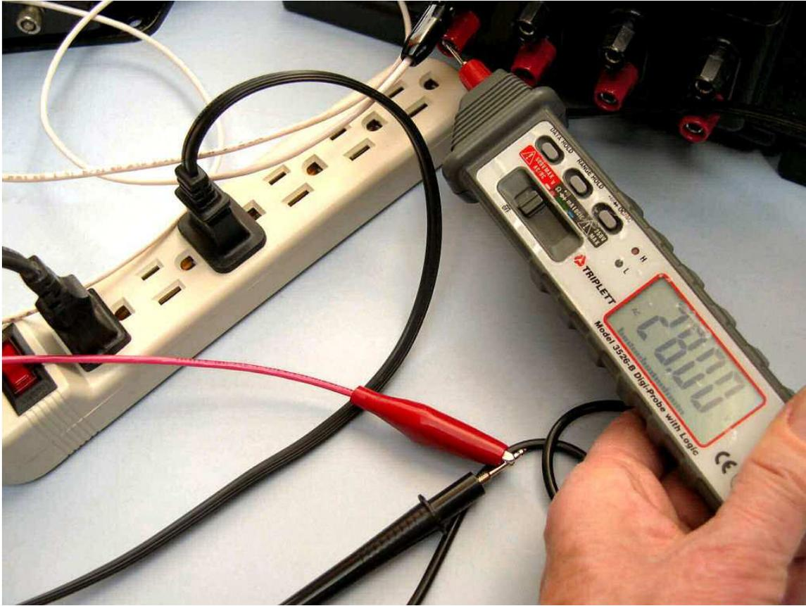
**Figure 4 – Voltage difference of 28 volts between out-of-phase transformers.**
