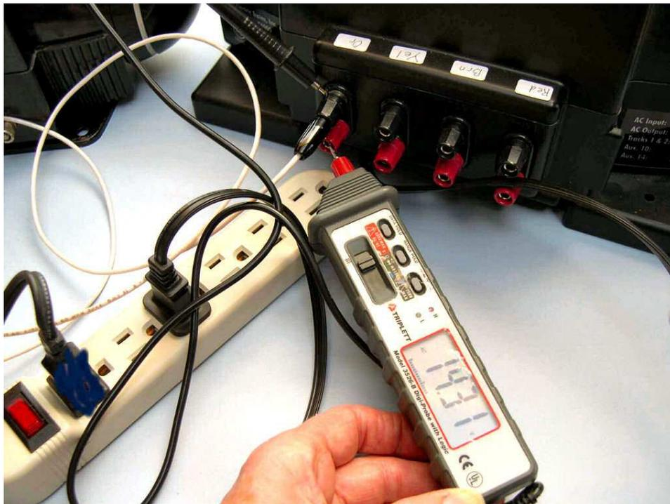
Figure 3 – Voltage output of a Z400 Transformer with throttle set at 14 volts
