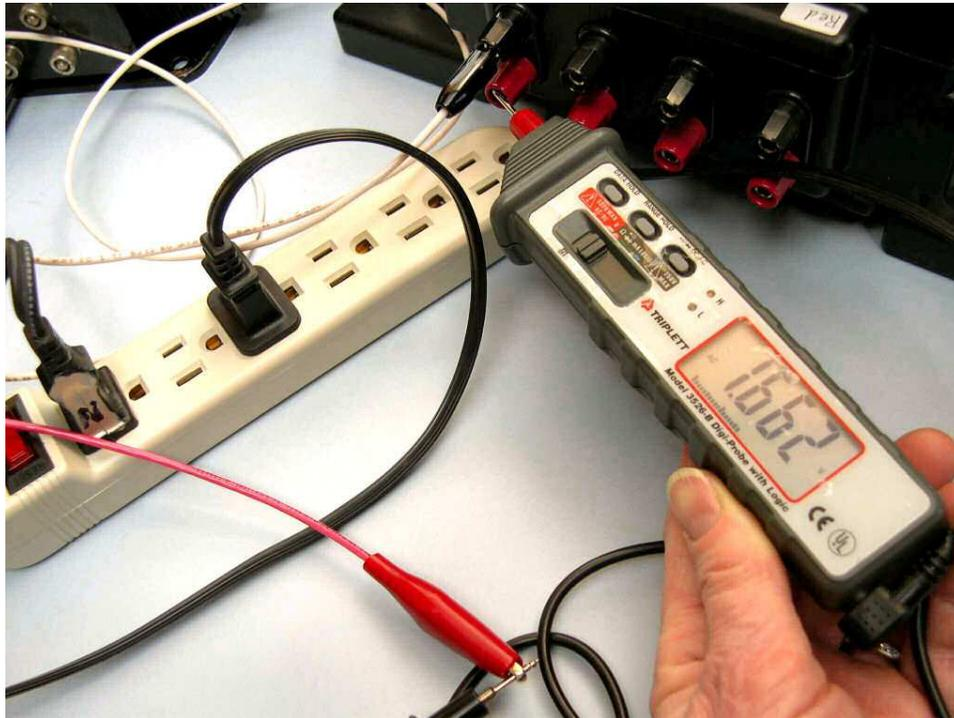
Figure 4 – Voltage difference of 1.662 volts between properly phased transformers.
