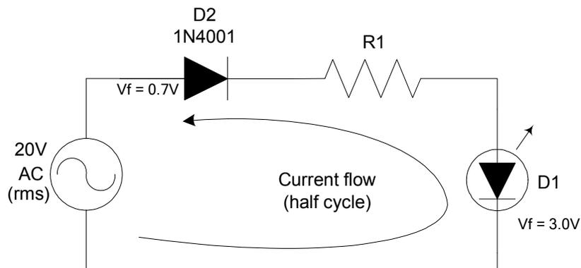
**Figure 5 – LED in an AC supplied circuit**
