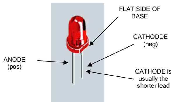
Figure 2 – LED packaging and lead identification
